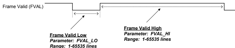
Figure 1-3: Frame Valid (FVAL) Timing Characteristics
